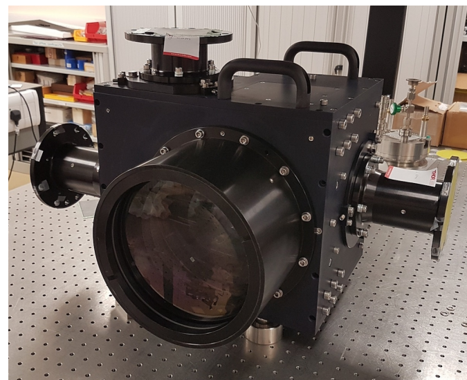
Left: The HiPERCAM hull, housing the four dichroic beamsplitters. The faces of the hull act as mounting points for the collimator and five re-imaging cameras – only three of the camera barrels are visible in this photo. The filter holders and CCD heads are mounted on the ends of the camera barrels. For scale, the large collimator lens visible in the photo has a diameter of 208 mm. Right: As-built transmission profiles of the HiPERCAM "Super" SDSS filters (solid lines), the HiPERCAM "original" SDSS filters (dotted lines), and the four HiPERCAM dichroic beamsplitters (dashed lines).
