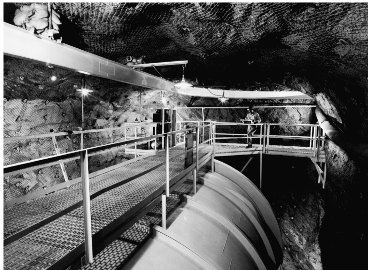
FIGURE 8 Raymond Davis's solar neutrino detector. The tank was located 1478 m (4850 ft) below ground in the Homestake Gold Mine in Lead, South Dakota, and was filled with 615,000 kg of C_2Cl_4 in a volume of 377,000 liters (100,000 gallons). (Courtesy of Brookhaven National Laboratory.)
