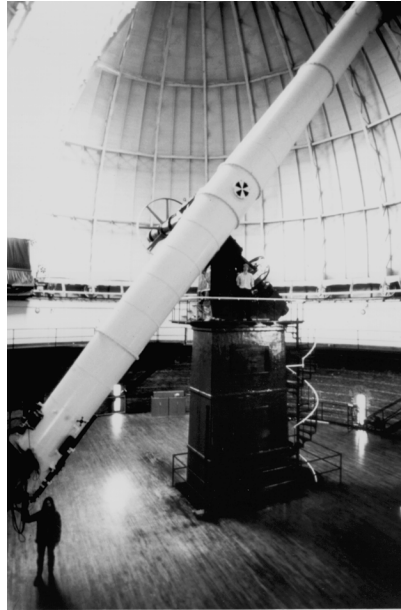
FIGURE 16 The 40-in (1.02-m) telescope at Yerkes Observatory was built in 1897 and is the largest refractor in the world. (Courtesy of Yerkes Observatory.)
