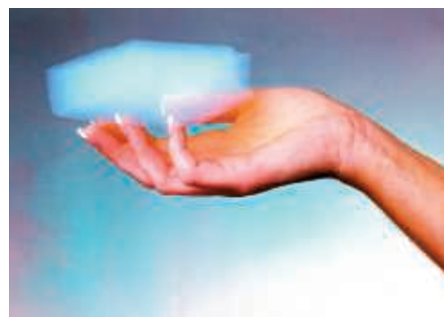
▲ FIGURE 4.12 Stardust at Wild-2 INTERACTIVE (a) The Stardust spacecraft captured this image (a) of comet P/Wild-2 in 2004, just before the craft passed through the comet's coma. (b) Onboard is a detector made of a foam-like jelly (called aerogel) that is 99.8% air, yet is strong enough to stop and store cometary dust particles as they hit the spacecraft. (c) Upon return of the craft to Earth in 2006, analysis began of the minute tracks in the aerogel, the ends of which contain captured comet dust fragments. (NASA)
