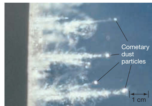
▲ FIGURE 4.12 Stardust at Wild-2 INTERACTIVE (a) The Stardust spacecraft captured this image (a) of comet P/Wild-2 in 2004, just before the craft passed through the comet's coma. (b) Onboard is a detector made of a foam-like jelly (called aerogel) that is 99.8% air, yet is strong enough to stop and store cometary dust particles as they hit the spacecraft. (c) Upon return of the craft to Earth in 2006, analysis began of the minute tracks in the aerogel, the ends of which contain captured comet dust fragments. (NASA)
