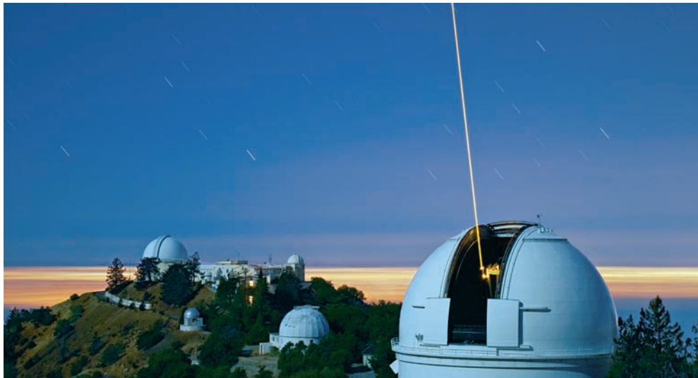
◀ FIGURE 5.19 Adaptive Optics System In this daytime photo, a test is being conducted at the Lick Observatory 3-m Shane telescope in California. A laser is used to create an “artificial star” (light reflected from the atmosphere back into the telescope) to improve guiding. The laser beam probes the atmosphere above the telescope, allowing tiny computer-controlled changes to be made in the shape of the mirror surface thousands of times each second. ( Lick Observatory )
