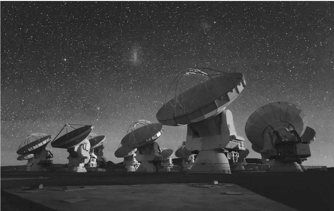
Fig. 3.31 The Atacama Large Millimetre Array (ALMA) built in cooperation by Europe, U.S.A. and Japan. The telescope has 64 antennas. (Photo ESO/NOAJ)
