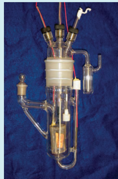
A laboratory cell for the investigation of cold fusion claims that were thereby found to be false.
