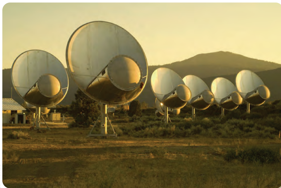
◀ Figure 26-13 Part of the Allen Telescope Array (ATA) near Mount Lassen in California, planned eventually to include 350 radio dishes, each 6 m in diameter, in an arrangement designed to maximize their combined angular resolution. Radio astronomers use the telescope to study galaxies and nebulae of astrophysical interest while SETI researchers employ state-of-the-art computer hardware and software to search for signals from distant civilizations.
