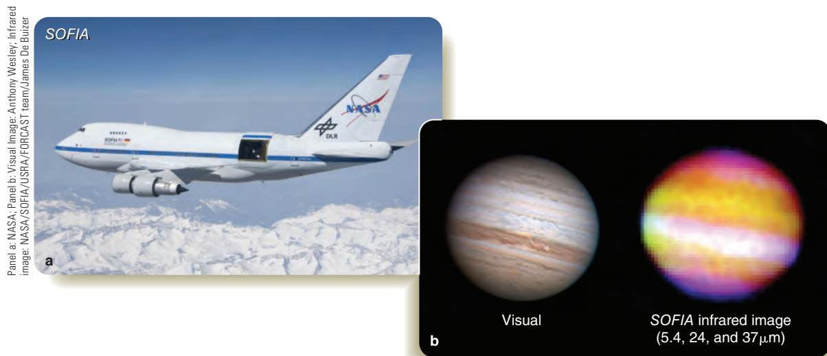
▲ Figure 6-18 (a) The Stratospheric Observatory for Infrared Astronomy ( SOFIA ), a joint project of NASA and the German Aerospace Center (DLR), flies at altitudes up to 14 km (45,000 ft) where it can collect infrared radiation with wavelengths that are unobservable even from high mountaintops. (b) A visual-wavelength image of the planet Jupiter ( left ) compared with a composite infrared image ( right ) using images at wavelengths of 5.4, 24, and 37 microns made during SOFIA 's “First Light” flight in 2010. The white stripe in the infrared image is a region of relatively transparent clouds through which the warm interior of the planet can be seen.
