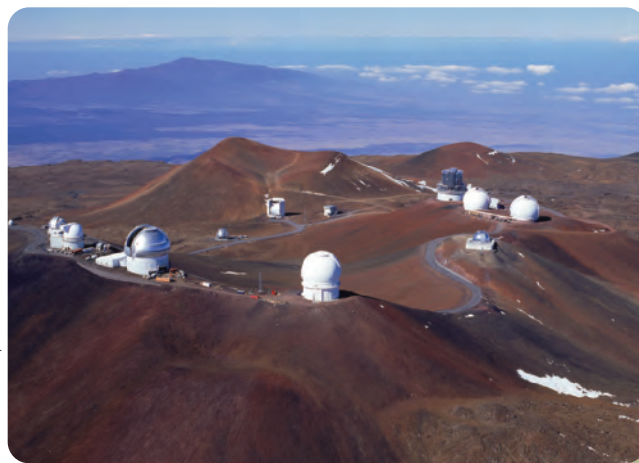
▲ Figure 6-13 Aerial view of the optical, infrared, and radio telescopes on Mauna Kea in Hawai’i, 4200 m (nearly 14,000 ft) above sea level. The high altitude, low atmospheric moisture, lack of nearby large cities, and location near the equator make this mountain one of the best places on Earth to build an observatory.
