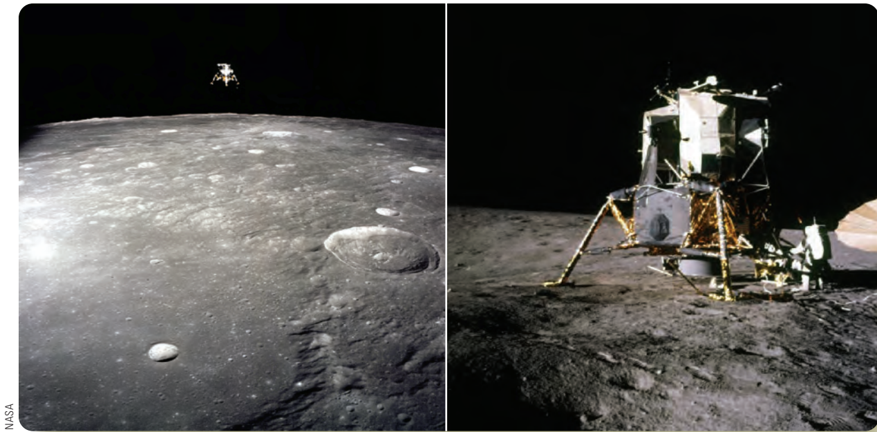
▲ Figure 21-3 Inside the lunar module, the two astronauts stood in a space hardly bigger than two telephone booths. The metal skin was so thin it was easily flexible, like metal foil, and the legs of the module, designed specifically for the Moon's weak gravity, could not support the lander's weight on Earth. Only the upper half of the lander blasted off from the surface to return the astronauts to the command module in orbit around the Moon.
