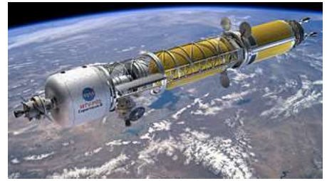
Concept for a Bimodal Nuclear Thermal Transfer Vehicle in low Earth orbit
