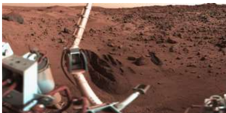
Viking 1 lander's sampling arm scooped up soil samples for tests (Chryse Planitia)
