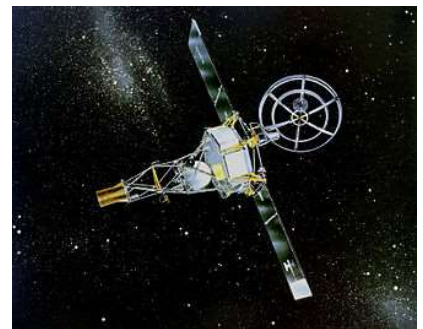
Artist's impression of Mariner 2 , launched in 1962, a skeletal, bottle-shaped spacecraft with a large radio dish on top
